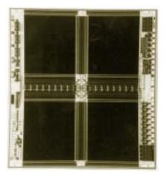
Radiation hardened 64-kilobit static random access memory chip from the early 1980s.
