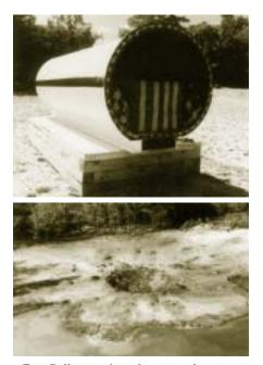
Fort Polk cratering phenomenology test conducted by DNA and U.S. Army Corps of Engineers to determine accuracy of Khobar Towers bomb damage assessment; upper photo is tank loaded with explosives, lower photo is resultant crater.
