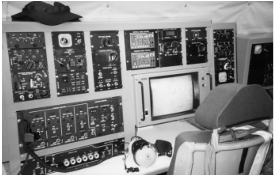
The video sensor control station on the OC-135B aircraft.
