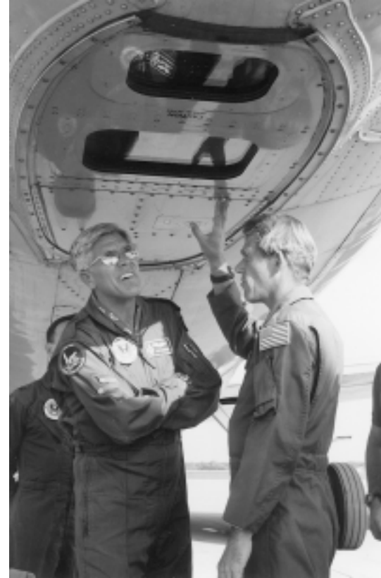
A view of the camera bay under the OC-135B.
