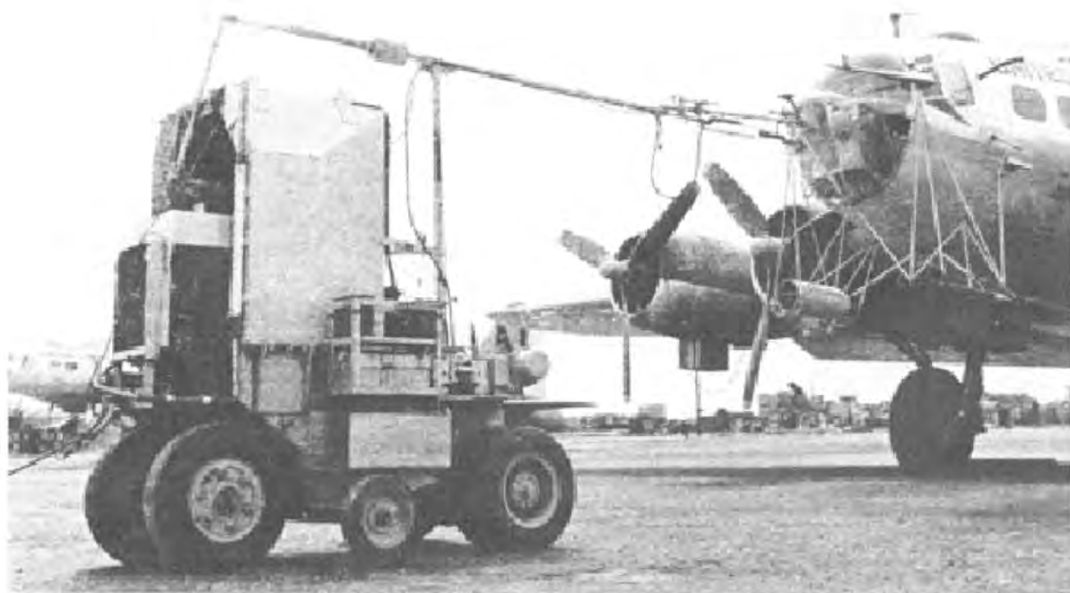
Figure 18. Removing gas sample from B-17 drone on Enewetak during GREENHOUSE.
