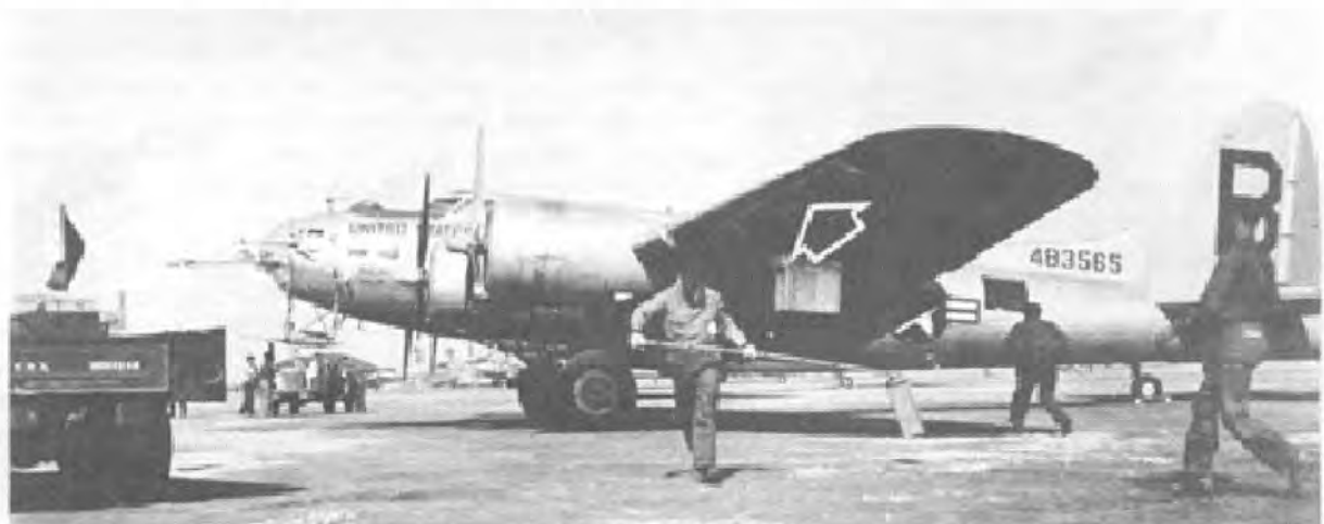
Figure 49. Contaminated panel recovery following GREENHOUSE, GEORGE. Arrow points to test panels taped on the underside of the wing.
